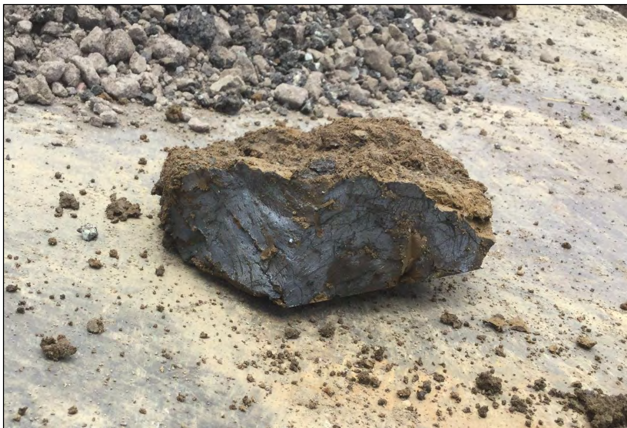
Figure 111. T-12 close-up of Stratum Ic clay with possible petroleum contamination
