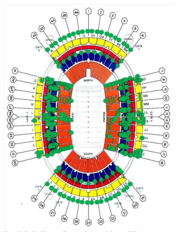
Figure 26. Graphical depiction of locations of recommended repairs: 2018 corrosion assessment
