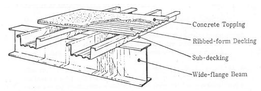
Figure 6. Schematic illustration of existing lightweight decking system at Aloha Stadium.
