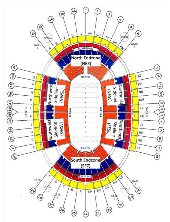
Figure 3. Exploded (colored sections not vertically stacked) plan view of the Aloha Stadium, indicating seating section letter identifiers and radial gridline numbering scheme.
