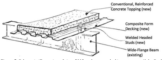
Figure 7. Schematic illustration of circa 2015 replacement decking system at Aloha Stadium.
