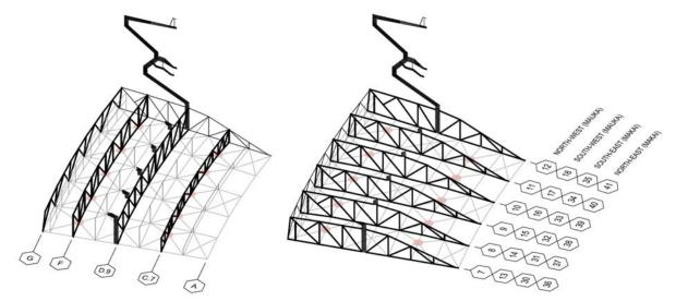
Figure 2. Schematic illustrations of the base truss system, located beneath the sideline seating stands, showing trusses along lettered transverse gridlines (left) separately from trusses along numbered radial gridlines (right).
